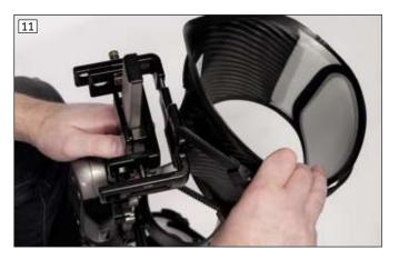
Set the adjustment unit with the thigh sleeve onto the frame structure.
