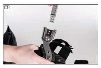
Mount the replacement base tube on the ankle joint with the two screws and tighten to a tightening torque of **6 Nm**.
