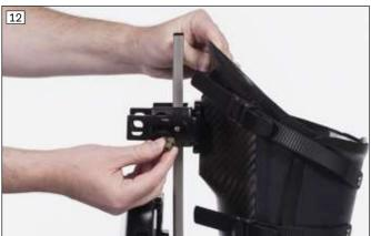
Put on the nut and tighten it with a **T 25** Torx wrench to a tightening torque of **4 Nm**.
