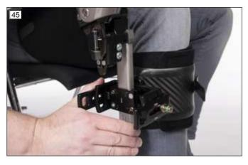
Slide the lower leg sleeve in the A-P direction until the laser points at the compromise pivot point.
