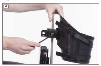
INFORMATION: The wrench symbol on the adjustment unit symbolises which of the two nuts must be removed and in what direction to pull off the unit.
