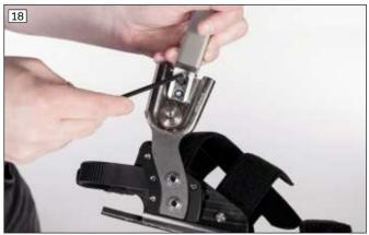
Loosen the two screws on the ankle joint with a **T 25** Torx wrench.
