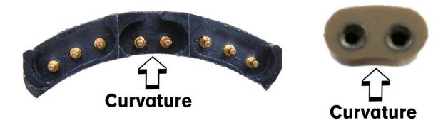
To avoid blowing a fuse in each Battery Pack inserted into the receptacle, match the slight curvature of the Plug to the curvature on the Controller. This is to be done when installing the Battery Cable into the 9E169 or 9E170 4-in-1 Controller.
