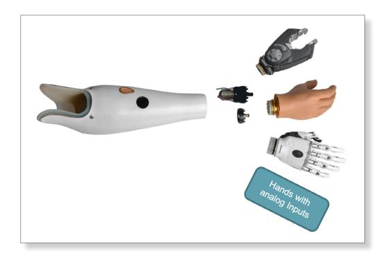
**Tech Tip:** Make sure the terminal device is connected to the prosthesis before powering on the system. If the terminal device is connected to the prosthesis after powering on, wrist rotation and open/close functions are active, but additional grip patterns of the bebionic hand cannot be recognized.
