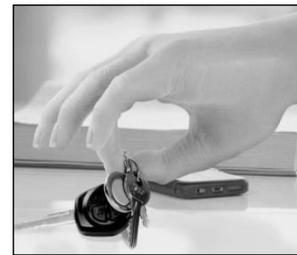
**13. Relaxed hand position** helps to give a natural and lifelike appearance. In the relaxed hand position, the thumb is positioned slightly towards the palm in the lateral position. The other fingers are slightly bent. By applying a further signal, the hand is moved into the hook grip for carrying objects.
