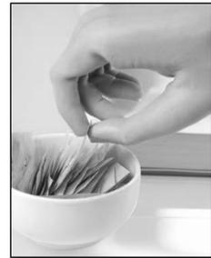
**10. Flexible Power grip** provides just the right amount of grip to suit any situation, whether shaking someone's hand, throwing a ball, using home and garden utensils or eating a piece of fruit. This grip pattern enables the user to hold round or cylindrical objects more easily and, above all, more securely.
